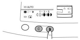
Set the number of copies using the copy quantity ((A), (A)) keys and press the print ((B)) key.
